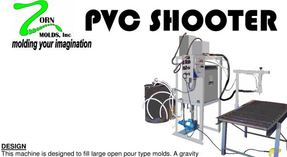
conveyor can be used to move your mold under the injector and fill the mold.
